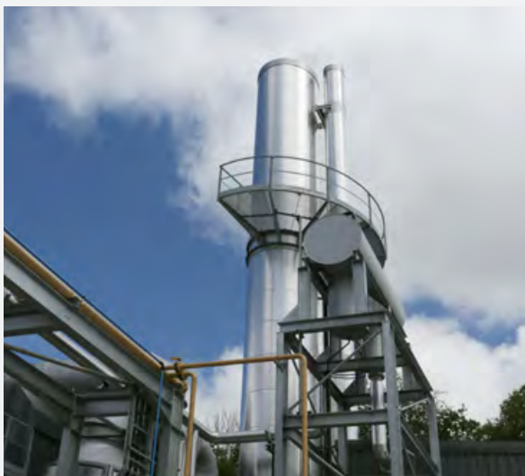
Our higher energy efficiency Regenerative Thermal Oxidiser in the Westhoughton site, which will reduce gas usage by an additional 30%.
